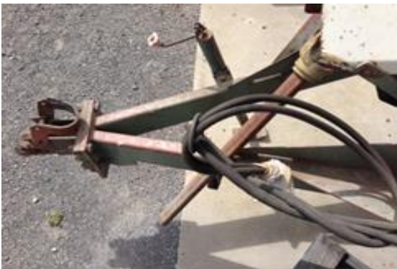
PTO guard missing
